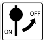
Fig. 22: Master switch of the hydraulic PTO shaft
