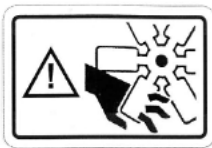
Fig. 19: Danger due to fan rotation
